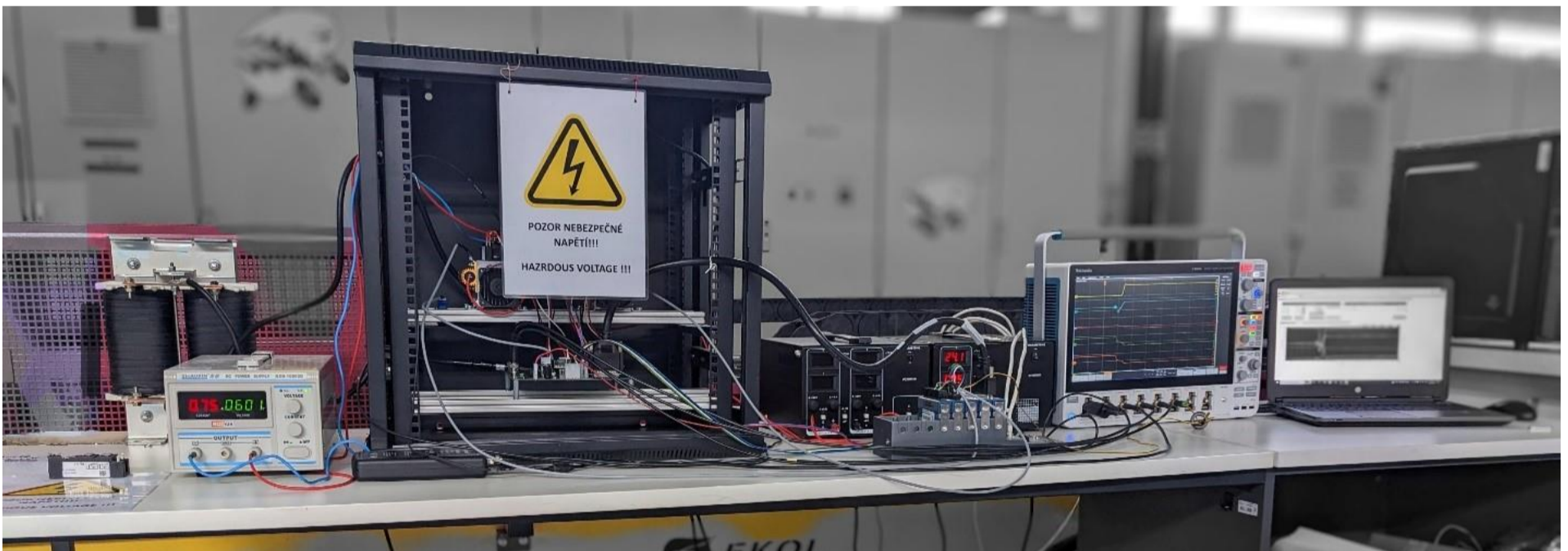
Fig. 1. The testbench setup for accelerated ageing tests of IGBT modules
